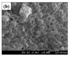
**Fig. 1** SEM micrographs of (a) the monodisperse hollow silica particles obtained by the two-step method and (b) the particles dried immediately after rapidly dissolving with acetone.
