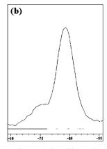
**Fig. 3** Solid-state <sup>29</sup>Si NMR spectra of monodisperse hollow silica particles. (a) The spectra of particles obtained after washing only with water. (b) The spectra of particles obtained after washing with ethanol three times.
