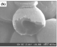
**Fig. 2** TEM micrograph of (a) monodisperse hollow silica particles (scale bar: 200 nm) and SEM micrograph of (b) the broken hollow particle after mechanically fracturing.
